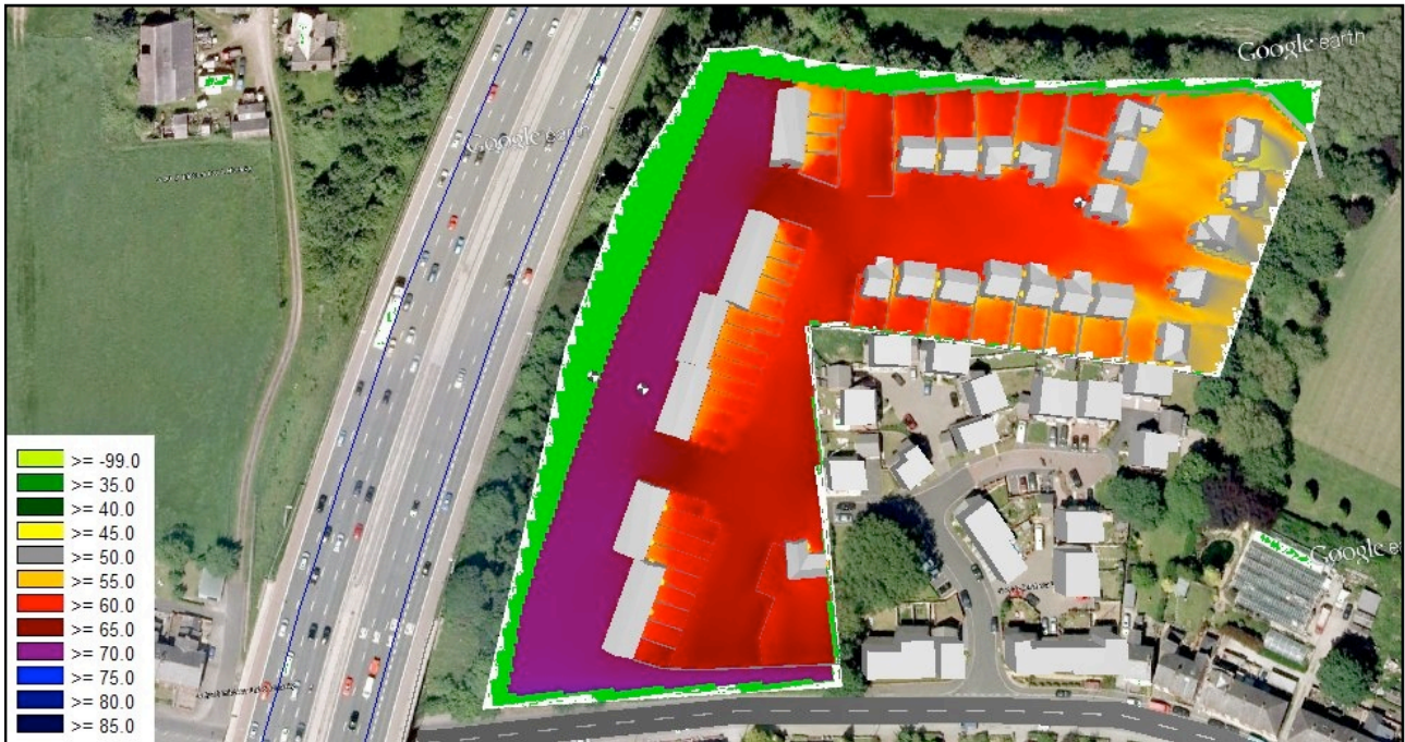
Figure 5: Predicted Daytime L_{Aeq} Propagation Across Site 1.5m (Ground Floor/Garden Level) - Proposed Site Plan
