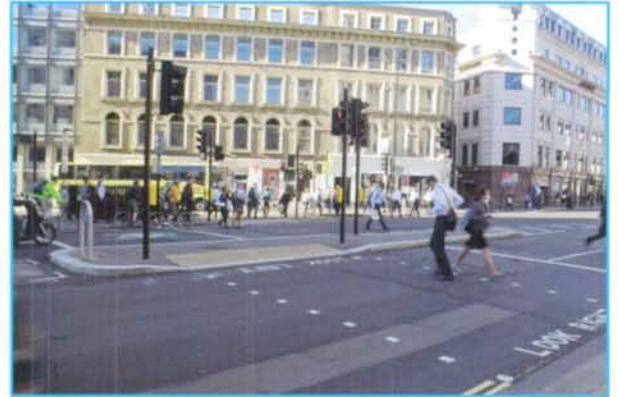
Staggered signalised crossing without guardrail
