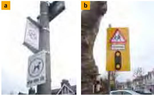
**Figure 9.1 (a) Sign clutter in residential areas; (b) the yellow backing board adds clutter and its use with the flashing amber lights is counter-productive. In addition, the sign post should not protrude above the sign.**
