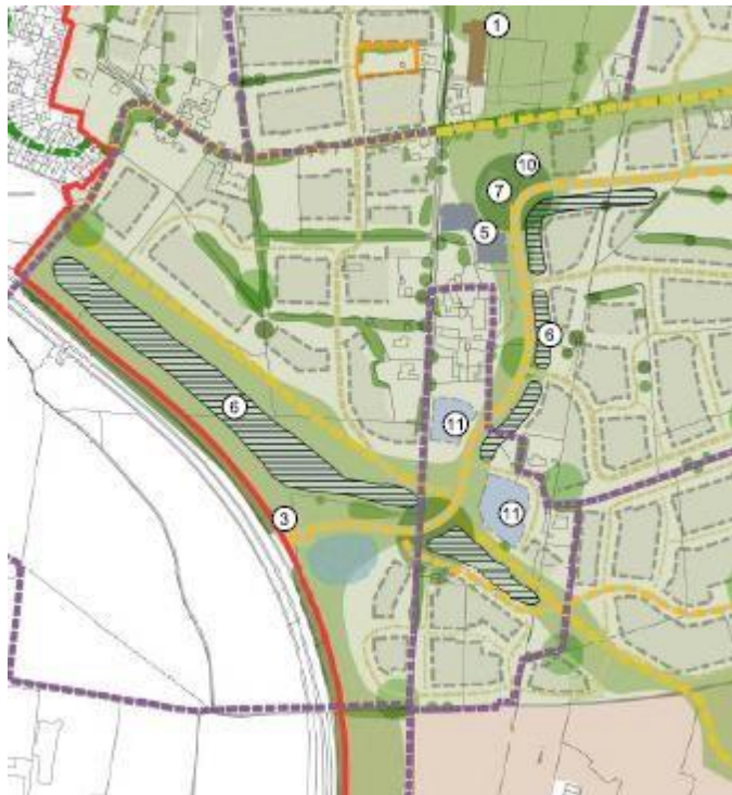
Catchment A attenuation ponds and swale system shown as feature 6.
